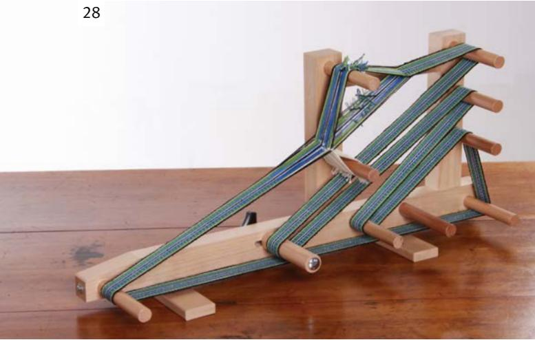
Stop weaving when you can't weave any longer because the knots in the warp are close to the leashes. You are now ready to remove your weaving from the loom BUT before you do, sew in the weft ends.
