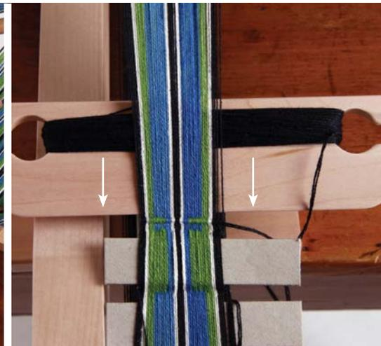
Pull the weft thread tightly. The warp threads will move together so you cannot see the weft at all through the warp.
