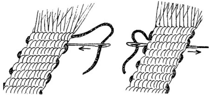
Sewing in weft ends. Sew the weft back three or four sheds to lock it, this is easier to do with the warp under tension.
