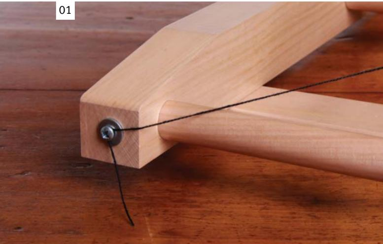
Wrap the beginning warp thread around the starter screw.
