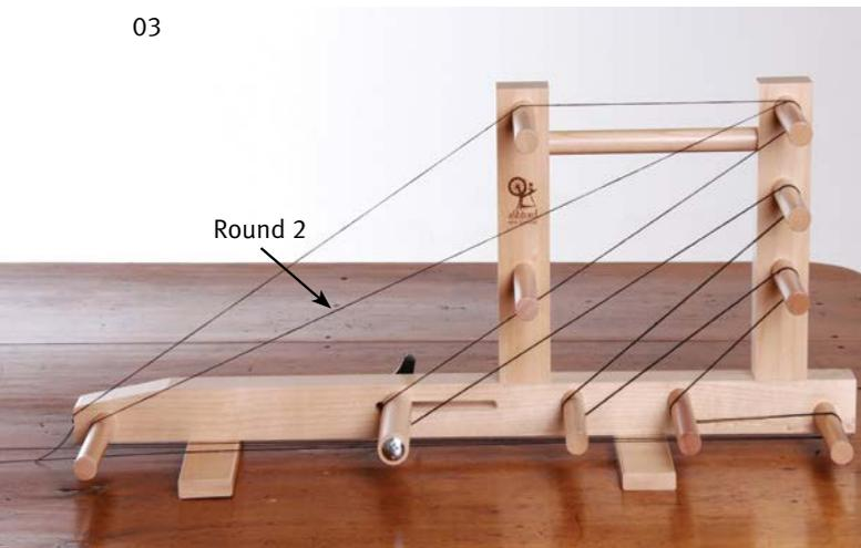
Round 2. Take the yarn straight up and over the top rear peg and around the same warping pegs and back to the starter peg. Repeat as per your draft.
