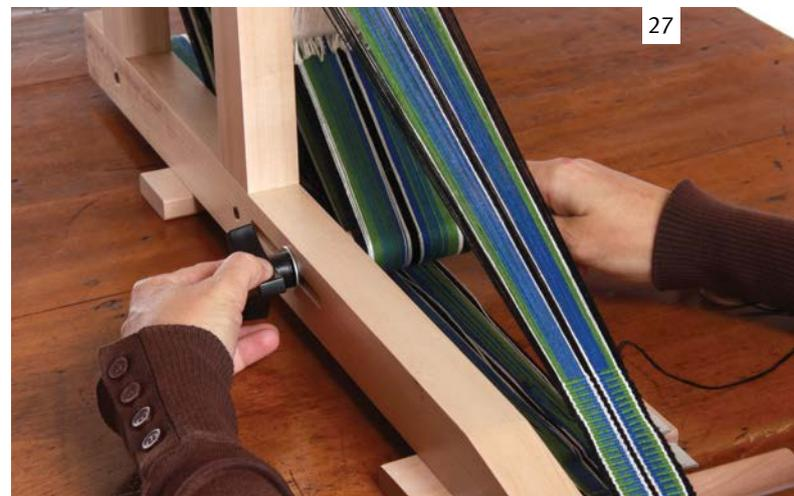
Pull the tension peg forward until the warp is tight. Tighten the nylon knob. As you move the weaving past the start peg you can remove the cardboard spacers. Continue weaving.
