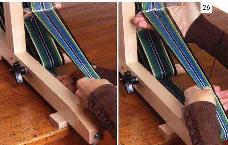
Gently pull the warp forward towards you until the end of the woven piece is about 5cm (2") from the front peg. All the threads will move around the pegs.
