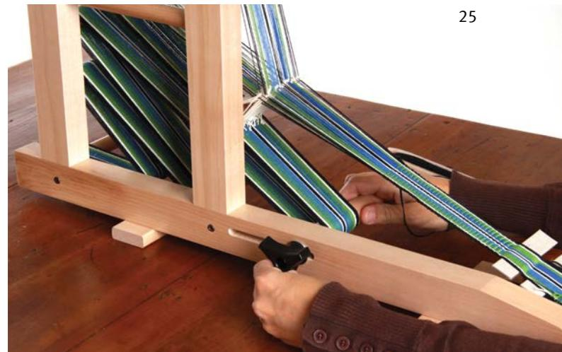
Winding on. Loosen the nylon knob. Move the tension peg back to loosen the warp.
