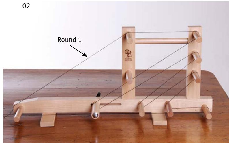
Round 1. Take the yarn up and over the top front peg and over top rear peg. Follow the warping pegs, including the tension peg and bottom peg and return to the starter peg.
