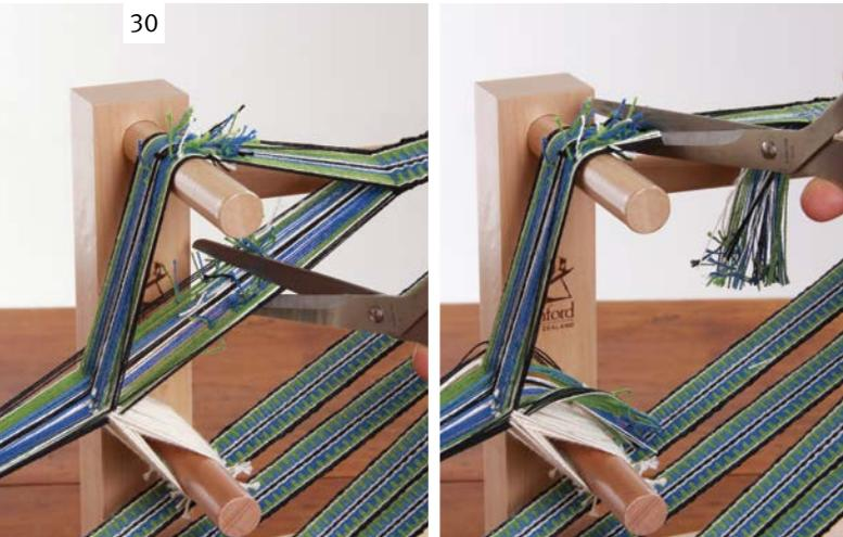
Remove the weaving from the loom by cutting each half of the warp a few centimetres (inches) behind the leashes. Pull the threads out off the leashes. To finish either let the ends hang loose as a fringe, plait them, twist them, tie knots in them or glue them and cut them close to the braid.
